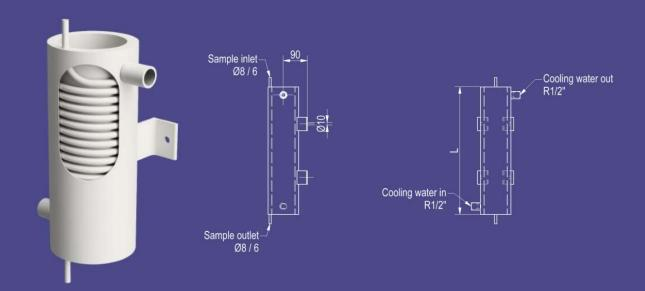
The VM sample cooler consist of two nested shells with water and a twisted coil between them. The shell material is stainless steel (EN 1.4307), and the sample cooling coil is made of stainless steel (EN 1.4404).
