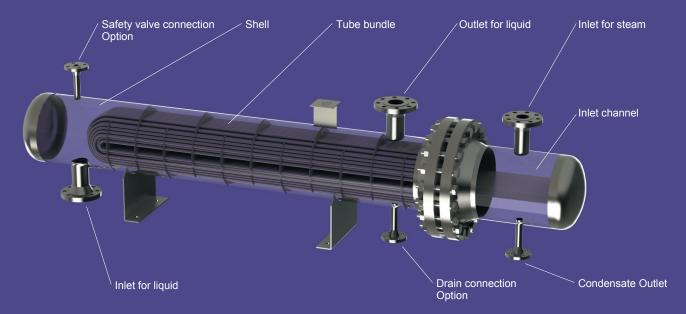
The diagram depicts the function principle of an oil/steam heat exchanger.
